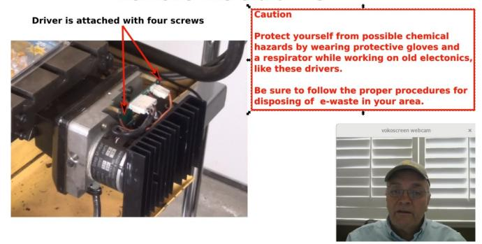
Next, remove the motor driver leaving the motor connectors behind. Beware of hazardous chemicals that may be present on the old motor drivers. I recommend wearing protective gloves and a respirator while removing the old drivers. Also be sure to properly dispose of the old motor drivers using the procedures established for e-waste disposal in your area.
