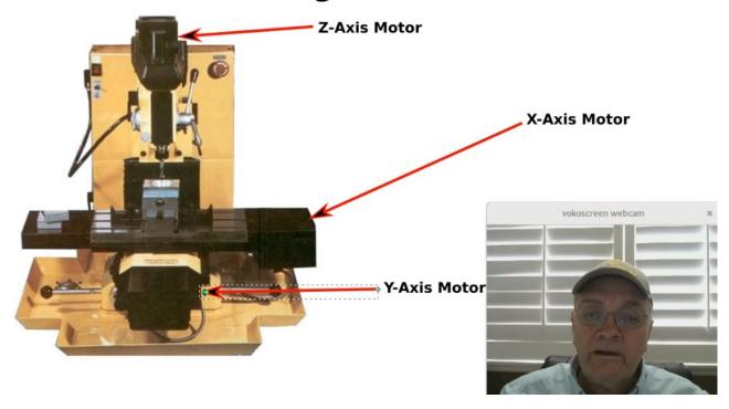
The motor on each axis must be connected to the respective port on the back of Buildbotics Controller.
