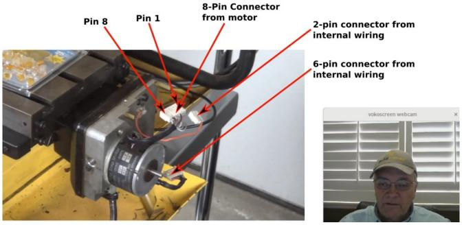
Three connectors are exposed after the motor housing and motor driver are removed. The eight pin connector comes from the motor. The six pin connector attaches to internal wiring that connects through the machine to the control cabinet. The two pin connector attaches to internal wiring that goes to the limit switches.
