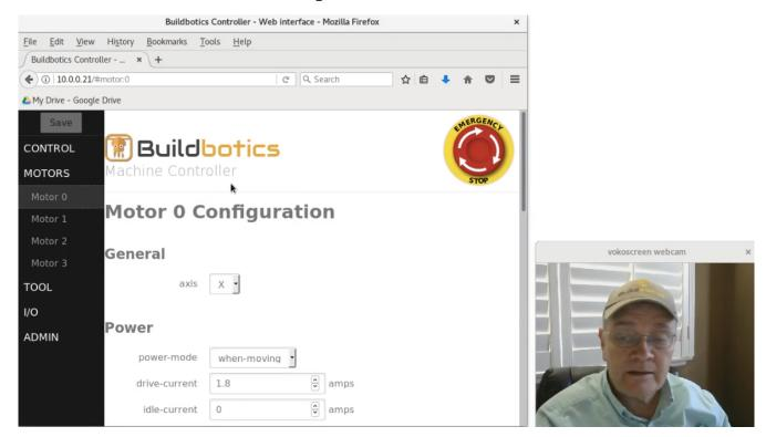
We'll start by configuring the X-axis motors and limit switches
