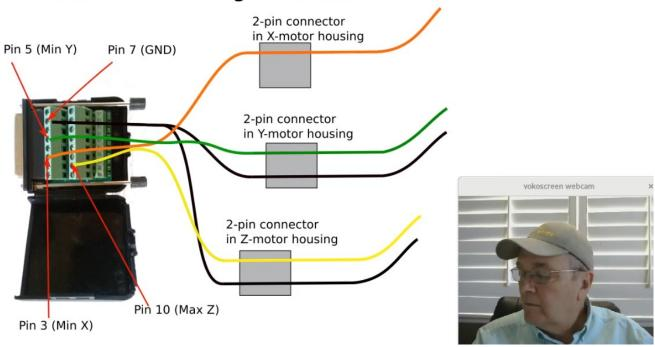
Limit switch wires are accessible inside the motor housing on the 2-pin connector. The connections for each axis are slightly different.
