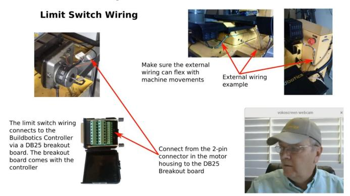
The limit switch wires extend from the 2-pin connectors inside the motor housing to the Buildbotics Controller via the DB25 breakout box that plugs into the back of the controller. The DB25 breakout box comes with the controller.
