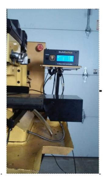
I recommend deciding where you want to locate the Buildbotics CNC Controller before starting to make electrical connections because the location of the new controller will determine how long the cables should be.
