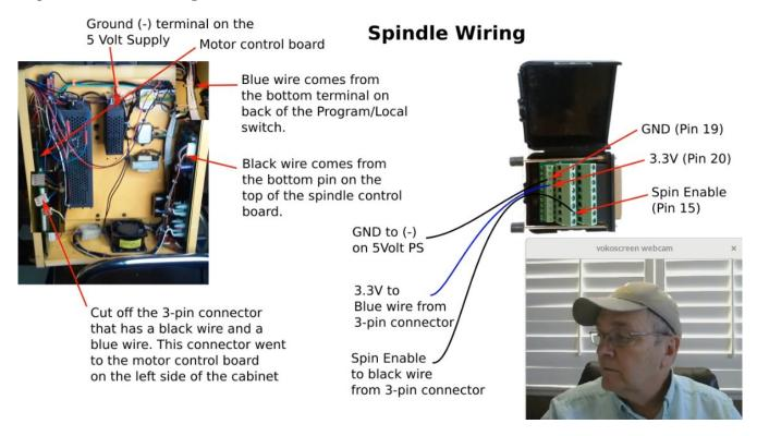
These connections will provide the ability to turn the spindle on and off from the Buildbotics Controller. The speed continues to be controlled with a rheostat on the side of the spindle.
