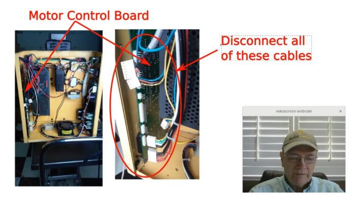
Make sure the Dyna is unplugged and turned off before removing the cover from the back cabinet to prevent exposure to hazardous electricity.
