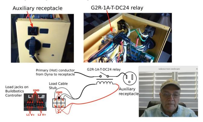
The user of the Dyna wants to use a coolant pump in conjunction with the Dyna. This diagram shows the circuitry required for controlling the auxiliary receptacle on the Dyna from the Buildbotics Controller.
