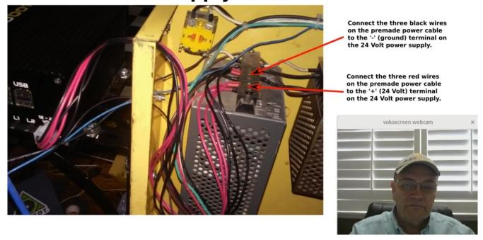
Connect the Buildbotics Controller to the existing Dyna 24Volt power supply using the pre-made power cable supplied by Buildbotics. Connect the three red wires to the plus terminal on the 24 Volt power supply inside the cabinet on the Dyna. And, connect the three black wires to the minus (or ground) terminal on the 24 Volt power supply. Plug the other end of the pre-made cable into the 12-36 VDC Power jack on the back of the Buildbotics Controller.
